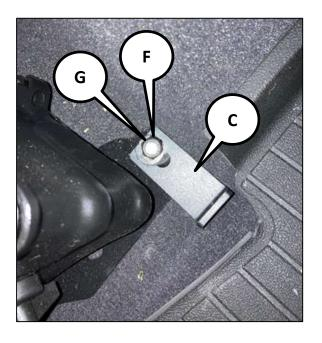
Install the rear seat storage drawer (A) in vehicle. Install bolts (D), washers (F), and nuts (E) through the box and then the brackets. Make sure the head of the bolt is inside of the box and the nut is on the outside of the box. Fully tighten the box to the brackets.
